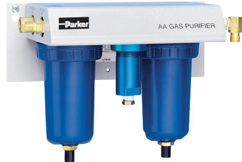
The purifier consists of two independent filtration systems. The first system is designed to purify the compressed air (oxidant) with two stages of high efficiency coalescing filtration. These filters will remove all oil, water, and particulate matter down to 0.01 micron.
