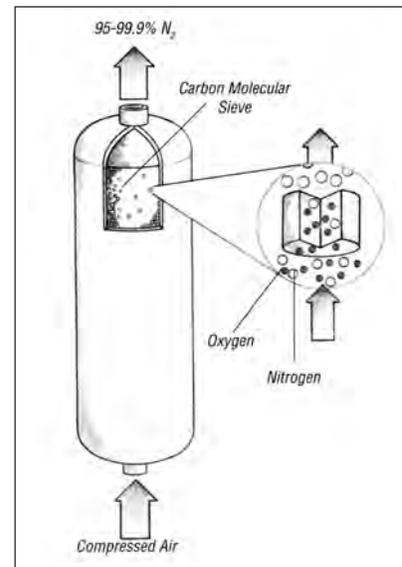
Pressure swing adsorption gas separation process adsorbs oxygen over nitrogen using carbon molecular sieve (CMS).
