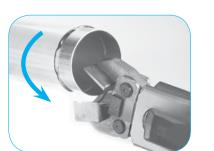
Re-open the two jaws to remove the pipe and rotate the pipe slightly.
